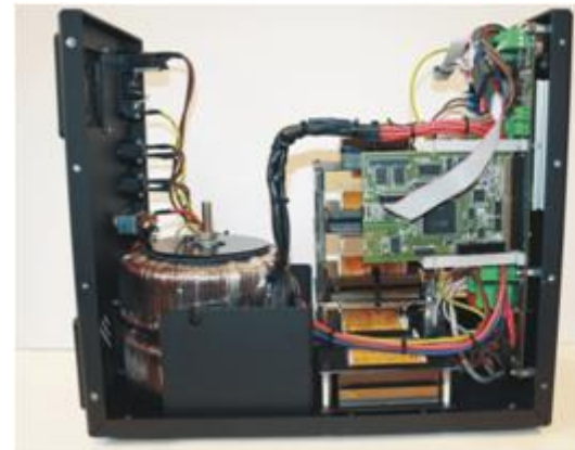
UPS for applications with special environmental exposures - including Li-ION battery module and BMS system
