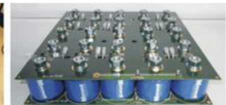
High power supply with output voltage backup after power failure and super capacitor module (16 F/ 60 V) with BMS system
