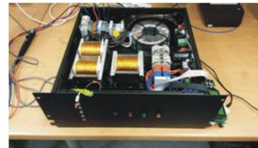
High power supply with output voltage backup after power failure and super capacitor module (16 F/ 60 V) with BMS system
