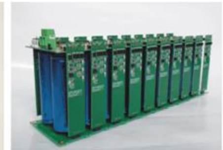
UPS for applications with special environmental exposures - including Li-ION battery module and BMS system
